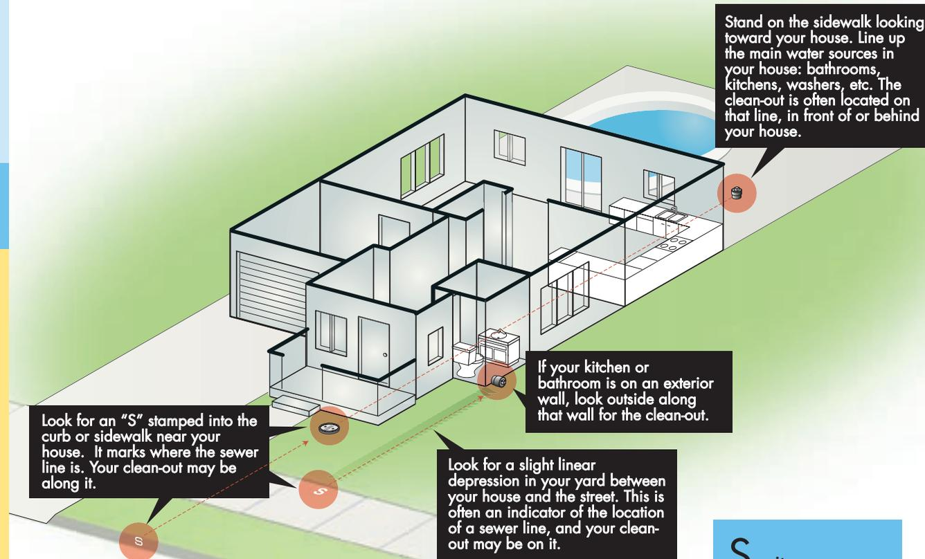
There are a number of places to look for your sanitary sewer clean-out. Start by checking to see if there's an "S" stamped into the concrete of your curb or sidewalk. This marks the location of the sewer line, and your clean-out may be aligned with this marking.
